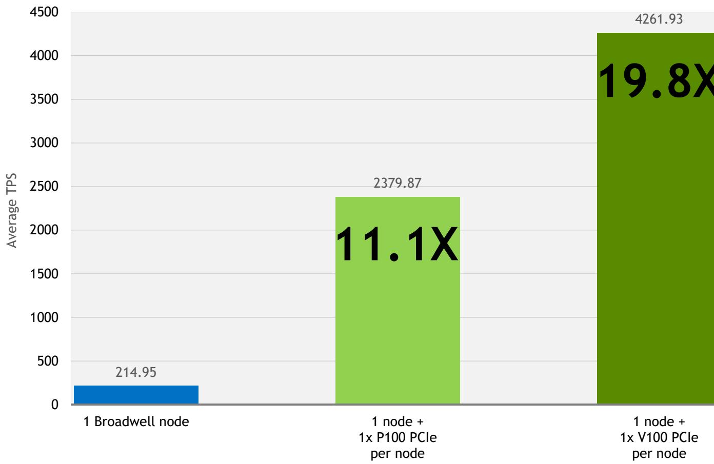
The **blue node** contains Dual Intel Xeon E5-2690 v4@2.6GHz [3.5GHz Turbo] (Broadwell) CPUs
