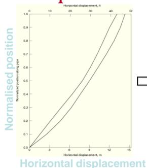
⇒ Displacement plot Vs riser position
