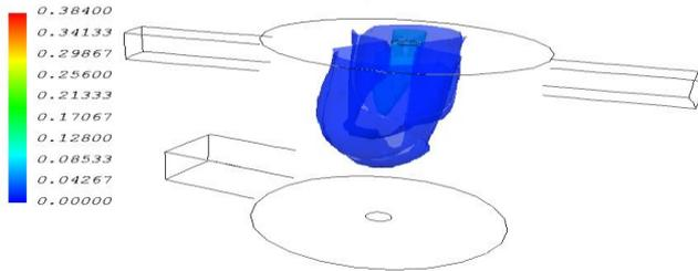
o Surfaces of NaCl Mass Fraction
