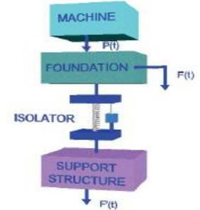
Free body diagram of the loads taken by the support structure
