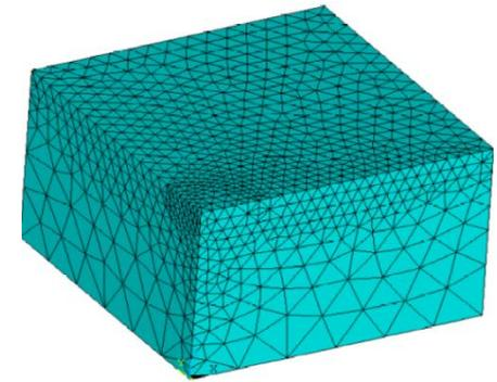
Finite element model of the foundation
