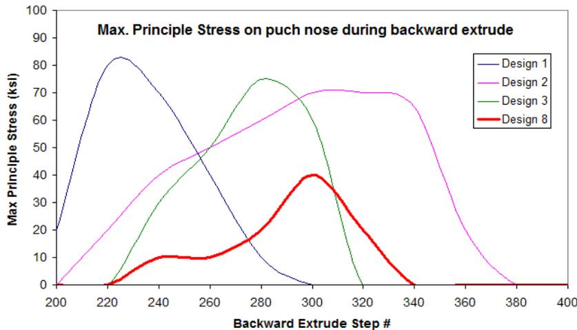
Successfully designed punch nose that has lower tensile stress during backward extrude
