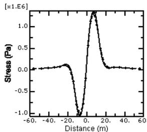
Axial stress along the bottom of the pipeline
